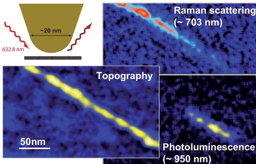
**Figure 1.** Topography of a DNA-wrapped single-walled carbon nanotube together with the simultaneously acquired near-field Raman and photoluminescence image. The spatial resolution of the optical images is about 15 nm.
