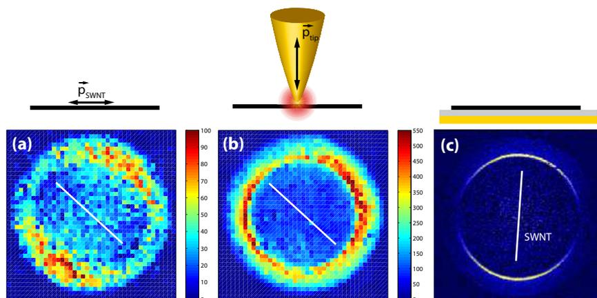
**Figure 2.** Angular photoluminescence radiation pattern detected from a single SWNT on glass without (a) and with metal tip (b). (c) Radiation pattern detected for a single SWNT deposited on a thin gold film. The radiation patterns indicate coupling to localized tip-plasmons in (b) and propagating surface plasmons in (c).
