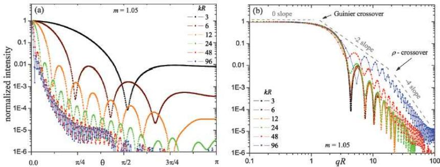
**Figure 1.** Power-law patterns for spherical particles. Plot (a) shows  $I(\theta)$  for particles with  $m = 1.05 + 0i$  and multiple size parameters  $kR$ . Plot (b) shows the *same* curves plotted as a function of  $qR$  along with the power-law envelopes and crossovers.
