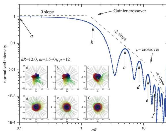
**Figure 3.** Scattered intensity for a spherical particle with  $kR = 12$  and  $m = 1.5 + 0i$  and corresponding color-coded phasor plots.
