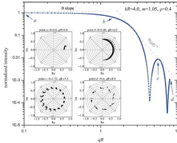
**Figure 2.** Phasor plots used to account for the power-law structure of  $I$  for a spherical particle with  $kR = 4.0$  and  $m = 1.05 + 0i$ .
