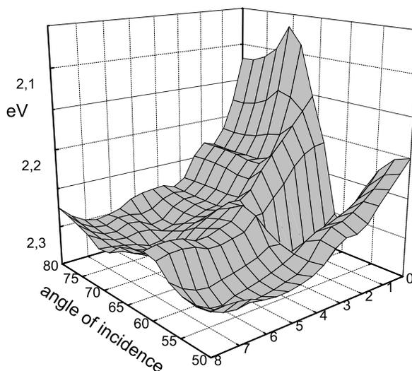
**Figure 1.** A The position of the resonance versus the angle of incidence and the mass thickness, which increases from  $N=8$  to  $N=0$ .
