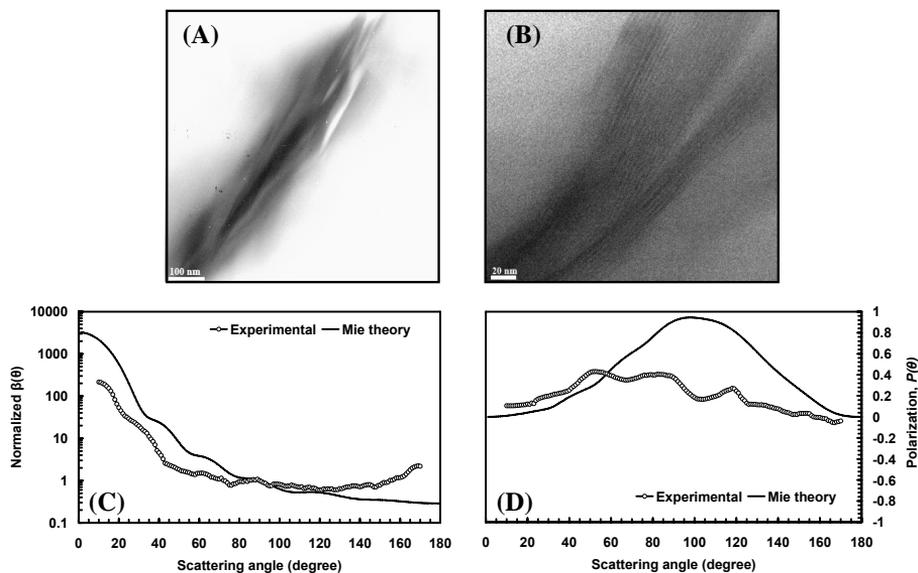
**Figure 2.** (A) TEM image of bentonite clay particle dispersed in the polymer matrix. (B) High resolution TEM image showing the typical layered structure (appearing as dark lines) of the bentonite clay particles. (C) Measured  $\beta(\theta)$  (dotted line) and (D)  $P(\theta)$  (dotted line) are compared with Mie calculations (bold line).
