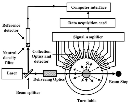
**Figure 1.** Schematic diagram of the light scattering setup (S: scattering centre).
