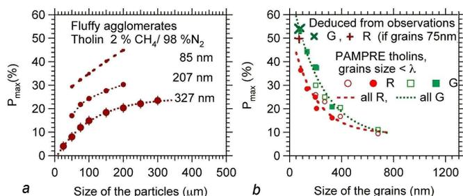
**Figure 4.** Amplitude of the positive branch vs sizes (a) of constituent grains (b) of agglomerates. Comparison to remote integrated observations on the whole atmosphere (extrapolated to the wavelengths used in the experiment).
