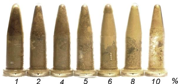
**Figure 2.** Decreasing darkness of the samples with increasing methane content in the gas mixture.
