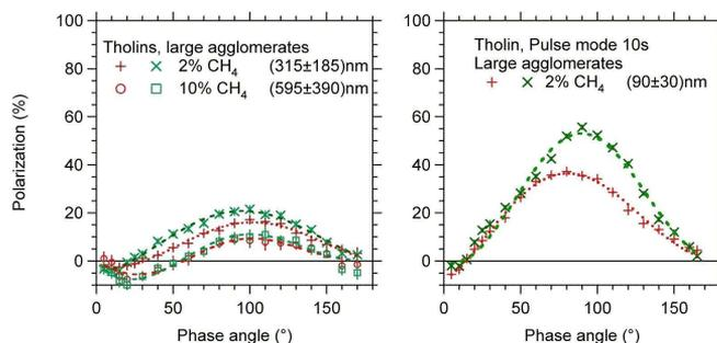
**Figure 3.** Polarization phase curves for 2 tholins at 2 wavelengths (543.5 nm and 632.8 nm)
