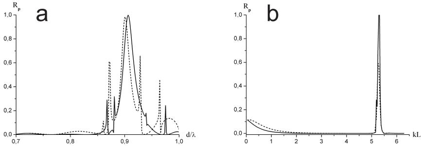
**Figure 1.** (a) The dependence of power reflection coefficient for the grating from identical layers. (b) The dependence of power reflection coefficient for hexagonal grating.
