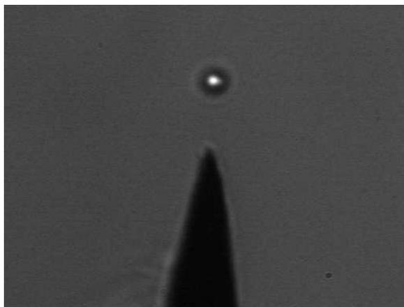
**Figure 1.** Optical microscopy picture of the charged trapped bead close to the electrode tip.
