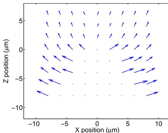
**Figure 2.** Electric field map around the tip shown in Fig.1. The tip is at the axis origin and the scanning step size is  $2 \mu\text{m}$ .
