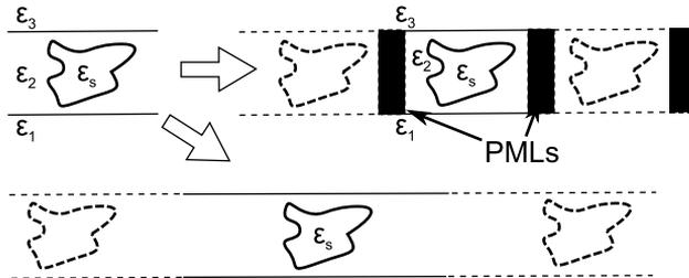
**Figure 1.** Two ways of transforming a non-periodic problem of the light scattering in planar media to a periodic problem of the light diffraction on gratings.
