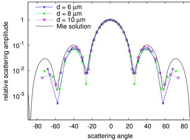
**Figure 2.** Comparison of the scattering diagrams obtained from the light diffraction calculation on a grating composed of spheres with the corresponding Mie solution.
