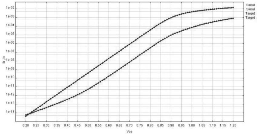
Fig. 2. Collector and base currents as a function of the base-emitter voltage. Dots represent target data while lines are simulated data (using extracted parameters and for null base-collector potential).
