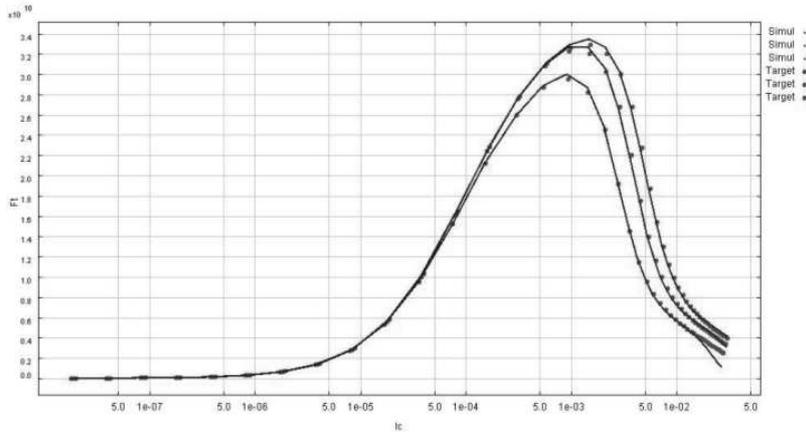
Fig. 1. Transition frequency as a function of collector current. Dots represent target data while lines are simulated data (using extracted parameters and for null base-collector potential).
