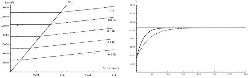
Fig. 1. Comparison of the solutions (7) (continuous line) with the experimental data by Swanson *et al.*<sup>11</sup>
