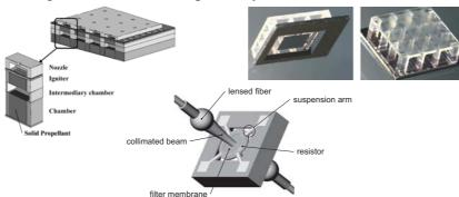
Fig. 2 MEMS case studies: microthruster (top left), gas sensor (top right), optical filter (bottom).
