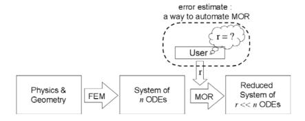
Fig. 5 Compact model extraction. Eliminating the need for user iteration makes the process fully automatic.
