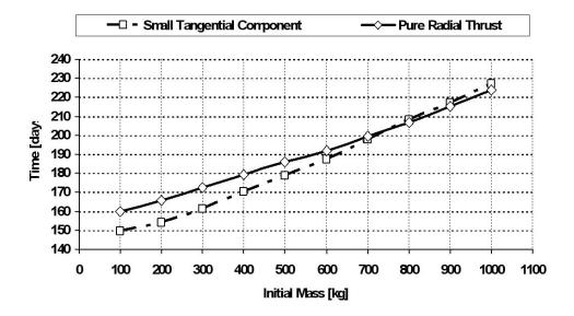
Fig. 2. Comparison between the transfer time vs the initial spacecraft mass, considering the two different thrust models. No relevant differences have been observed.
