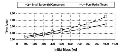
Fig. 6. Comparison between the escape time vs the initial spacecraft mass, considering the two different thrust models. No relevant differences have been observed.
