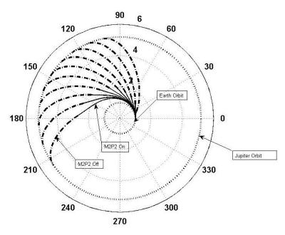
Fig. 3. Transfer trajectories towards Jupiter according to different values of the starting spacecraft mass, in the range 100 - 1000 kg. The dashed segments in the figure represent the trajectory arches where the M2P2 was active. Thrust is assumed to be along the radial direction.
