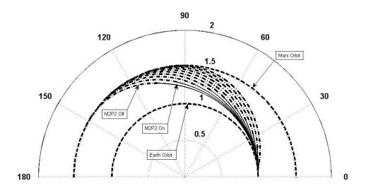
Fig. 1. Transfer trajectories towards Mars according to different values of the starting spacecraft mass, in the range 100 - 1000 kg. The dashed segments in the figure represent the trajectory arches where M2P2 was active. Thrust is assumed to be along the radial direction.
