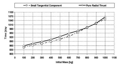
Fig. 4. Comparison between the transfer time vs the initial spacecraft mass, in the range 100 - 1000 kg, considering the two different thrust models. No relevant differences have been observed.
