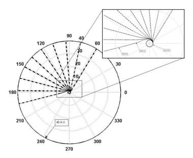
Fig. 5. Escape trajectories according to different values of the starting spacecraft mass, in the range 100 - 1000 kg. The dashed segments in the figure represent the trajectory arches where the M2P2 was active. In the enlargement, the early phase of the transfer.
